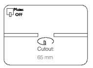
Choose the location of your new downlight, giving consideration to joists, water pipes, wiring or any other obstacles that may hamper installation. Please also ensure you have adequate ventilation and/or ceiling clearance in the relevant voids. Using a hole cutter, cut the appropriate cutout for the downlight.
