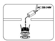
Feed cables thorough and make the electoral connections to the led driver according to relevant regulations in your territory.
